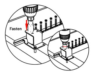
• Rotate the tool away from the board using the screw located against the joist as the pivot point. The action will tear the installed clip from the remaining collation. Slide the collation down the tool so the next clip is ready to install, and repeat.
