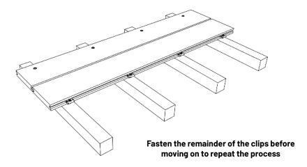
**Note:** It is essential not to over-tighten any fixing before the next board has been clipped in and secured. Previously installed clips can be tightened, but it is important to do this after the next row of clips has been installed to prevent the recently clipped in board from being pushed out of place.
