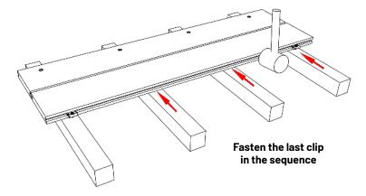
• Fasten the remainder of clips between the first and last clip ensuring the board is correctly positioned relative to the previous row clips.
